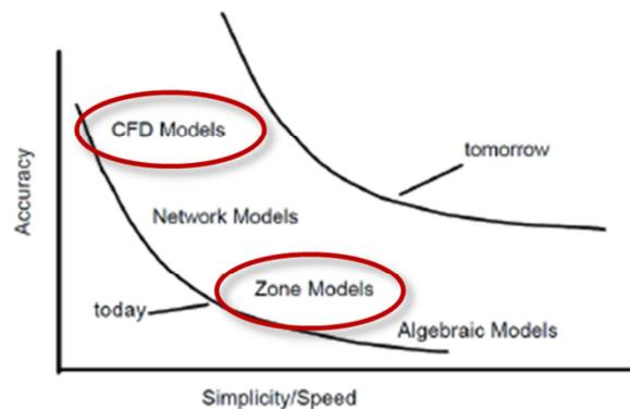
Figure 1: Hierarchy of fire simulation models <sup>3</sup>
