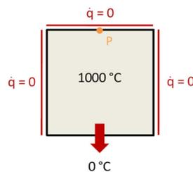
Figure 3: Mock-up for the example from the National Annex of EC 1-1-2<sup>6</sup>
