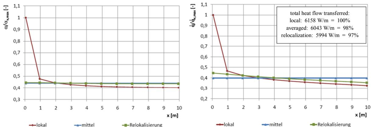
Figure 10: Distribution of the heat transfer coefficient and of the convective heat flux along the duct (normalised) – “heating of the fluid“
