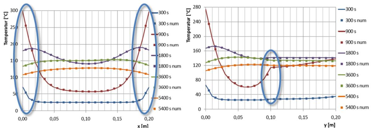
Figure 5: Results with convective and radiative heat transfer
