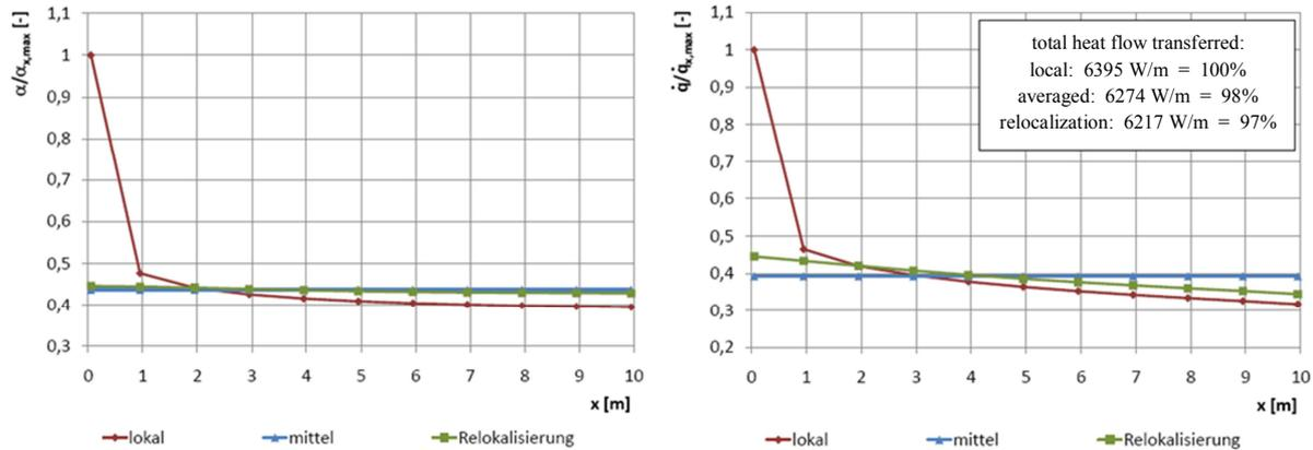
Figure 11: Distribution of the heat transfer coefficient and of the convective heat flux along the duct (normalised) – “cooling of the fluid“
