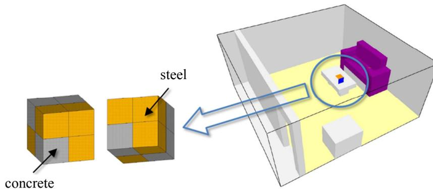
Figure 4: Realistic fire scenario of a room fire in FDS5
