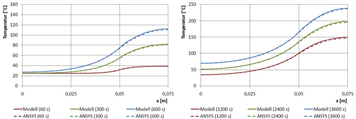
Figure 9: Results with a heat source in the style of a pyrolysis model
