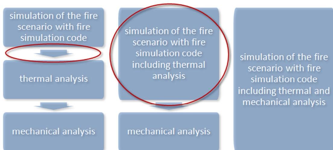
Figure 12: Modus operandi for the structural fire design in combination with natural fires
