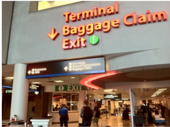
Figure 12. Charlotte-Douglas Intl. Airport. Large open spaces with unclear exit paths. Ambiguous exit signage. It is not clear where the emergency exit is located and how long is the emergency exit path (e.g.: do the evacuee have to go though the terminal and the baggage claim to finally find the exit?).
