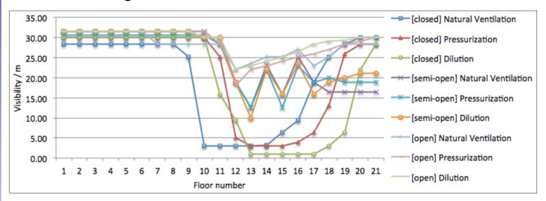
**Pressurization system** – exerting a pressure that prevents the smoke from entering the stairwell, so the visibility is:
