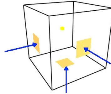
Figure 8: *scarc3d*-geometry with steadily changing inflows from three sides
