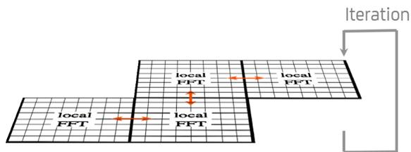
Figure 6: Multi-mesh FFT with additional averaging iteration for the 2D pipe geometry
