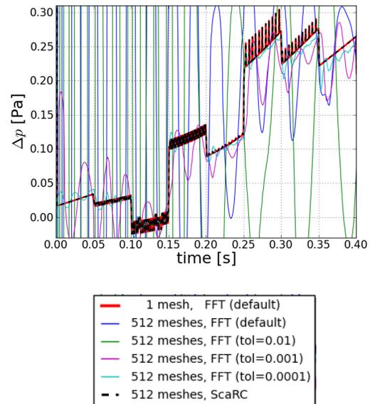
Figure 11: Comparison of the pressure devices for the 512-mesh cases against the 1-mesh case
