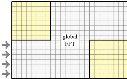
Figure 3: Single-mesh discretization with global FFT-method for the 2D pipe geometry
