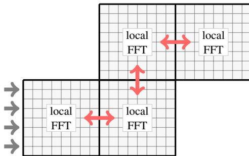
Figure 4: Multi-mesh discretization with local FFT-methods for the 2D pipe geometry
