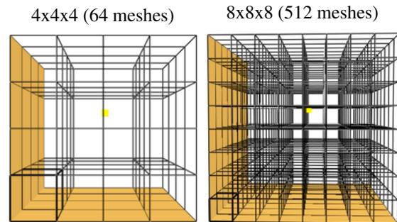
Figure 9: 64- and 512-mesh decomposition for the 'scarc3d'-case
