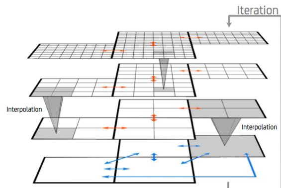
Figure 7: Geometric multigrid variant of ScaRC with different grid levels
