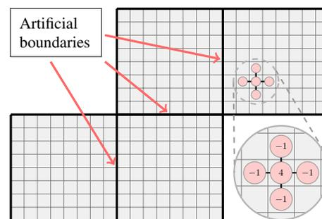
Figure 2: Discretization of a 2D pipe geometry with 5-point matrix stencil
