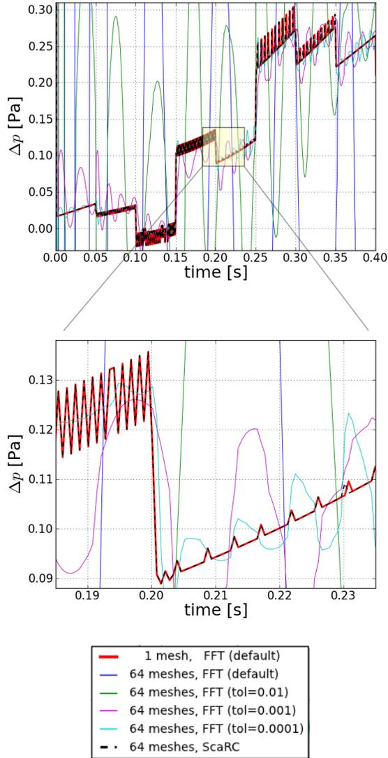
Figure 10: Comparison of the pressure devices for the 64-mesh cases against the 1-mesh case
