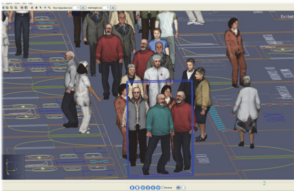
Figure 5 bottleneck in the smoke proof enclosure
