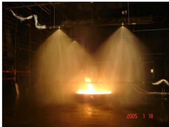
Figure 11. Sprinkler activation during the experiment. [19]
