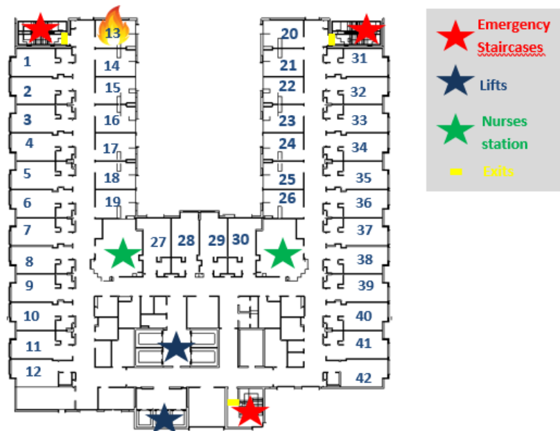
Figure 1. Layout of the 6th floor of the G bloc of the Clinique Sainte Elisabeth
