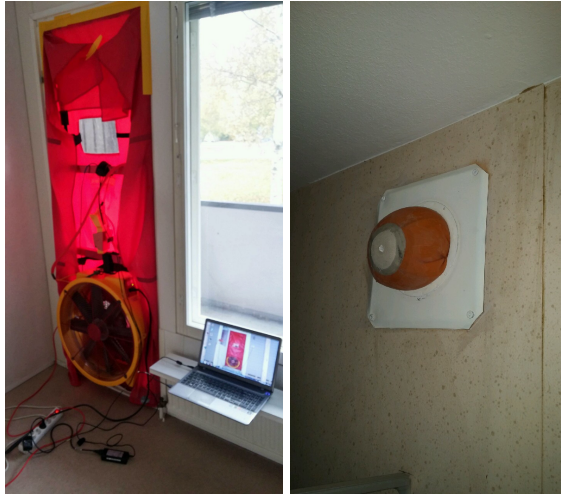
Figure 1. Blower-door test (left) and sealed exhaust ventilation duct (right). (Photographs by Mikko Yli-Piipari, Vertia Oy).
