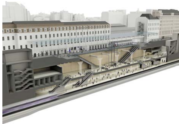
Figure 2.a- – Cut & Cover station of Crossrail Paddington station in London (I).
