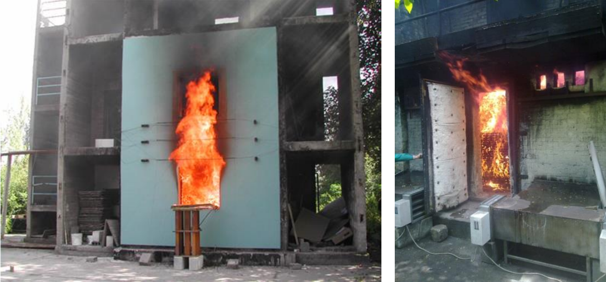
Figure 1-2: Facade test on fire propagation seen from the front and from the back, the side of air supply openings
