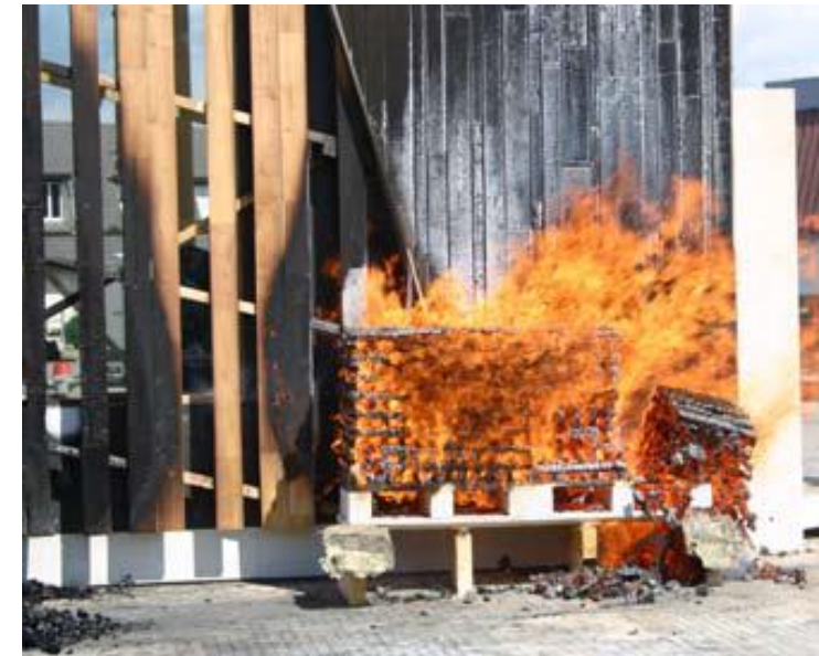
ÖNORM B 3800-5 – medium-scale test External fire exposure
