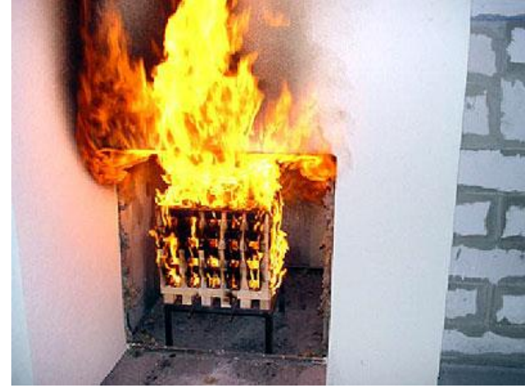
ÖNORM B 3800-5 – medium-scale test External fire exposure
