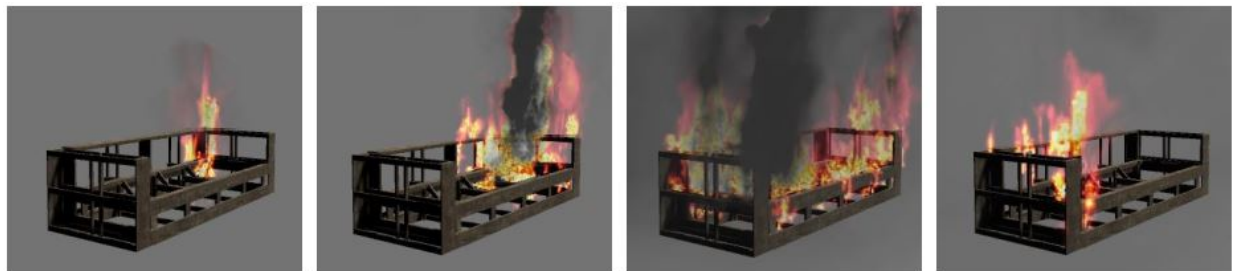
Figure 8: Burning couch frame at time frames t=5s , t=60s , t=210s and t=290s
