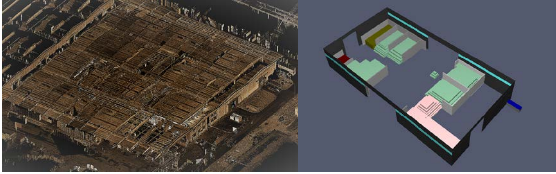
Figure 1: Point Cloud from laser scanning (left side) and 3dModel in PyroSim (right side).
