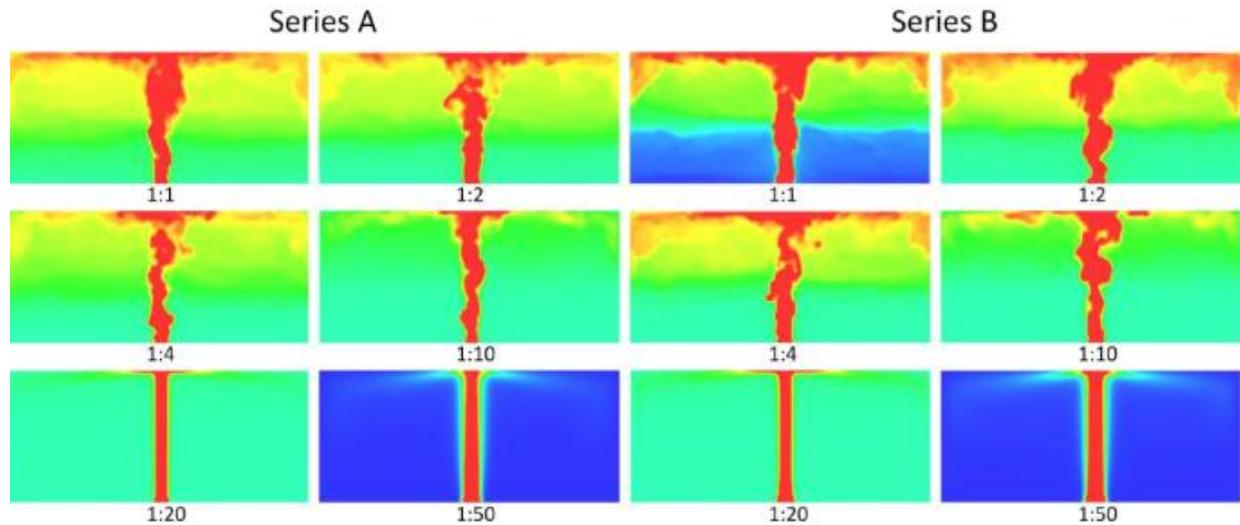
*Figure 10. Temperature slice through the centerline of the smoke plume, with visible vortices forming in the plume and laminar structures in scales 1:20 and 1:50. The color scale was individually altered to illustrate the flow structure of the plume*
