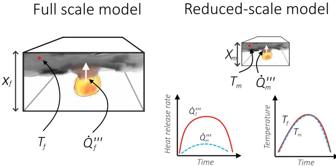
Figure 1. The idea of the Froude-number reduced-scale fire modelling. Illustrating the concept of scaling down the heat release rate of the fire to model a fire, that causes similar consequences in the scaled down (geometrical) compartment [5]
