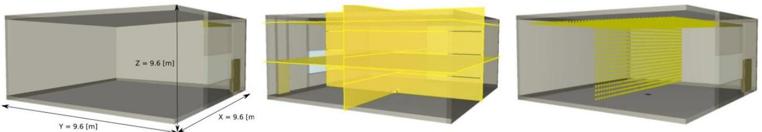
Figure 4. Full- 3-D model of the laboratory in full scale and the arrangement of 2D-slices and measuring devices used in the result analysis
