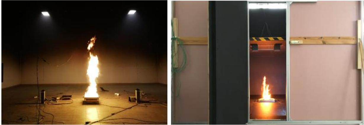
Figure 3. Full-scale (left) and small-scale (1:4)(right) experiments on the free burning of n-heptane [5]
