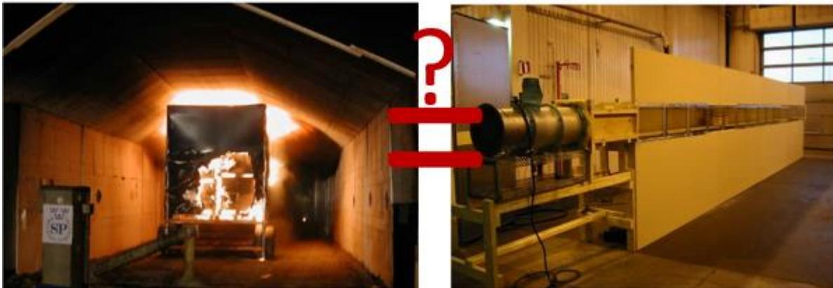
Figure 2. Two fire experiments in different scales representing the same fire. The left picture shows a photo from Runehamar tunnel fire tests [8]. The right photo shows 1:23 model-scale representation of these tests [7]
