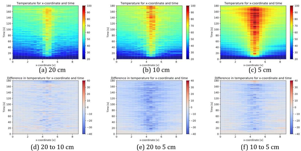
Figure 5. Comparison of results of mesh sensitivity analysis for maximum values of centerline plume temperature (a-c), and the difference between each of the grid size (d-f)
