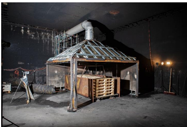
Figure 2 Photo of the calorimeter and the mock-up equipped with the fire load used during fire test. ©FOGTEC
