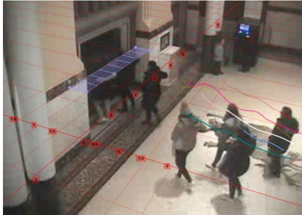
Figure 2: Kinovea tracking person movement with surveyed grid (Gales et al., 2022) (Young and Gales, 2022) Note: the airport video footage is not shown at this stage as currently non-disclosure agreements specify that footage from the surveyed days cannot be reproduced in publication.
