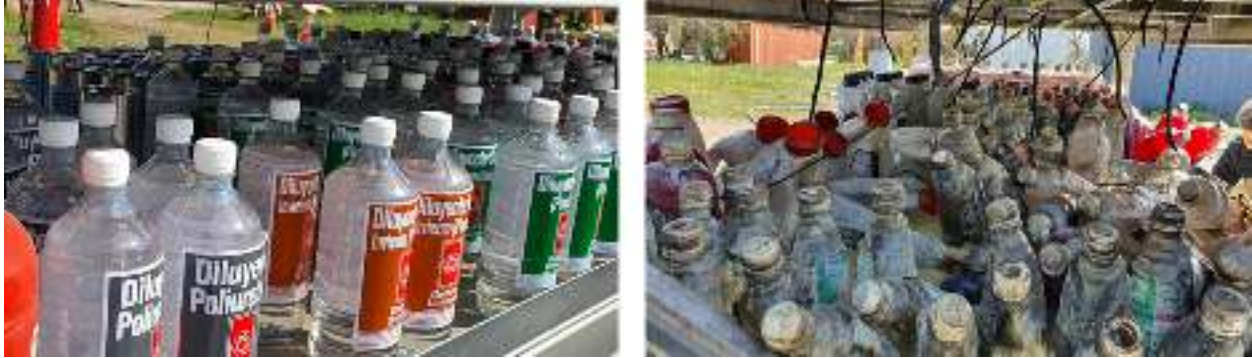
Figure 12: Left, bottles before fire – Right, bottles after fire
