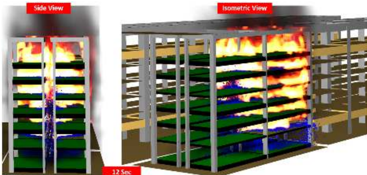
Figure 28: Simulation after 12 seconds from ignition
