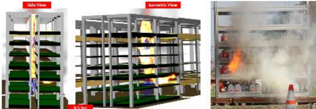
Figure 35: Comparison of Fire Simulation (Left) and Real full-scale test (Right)
