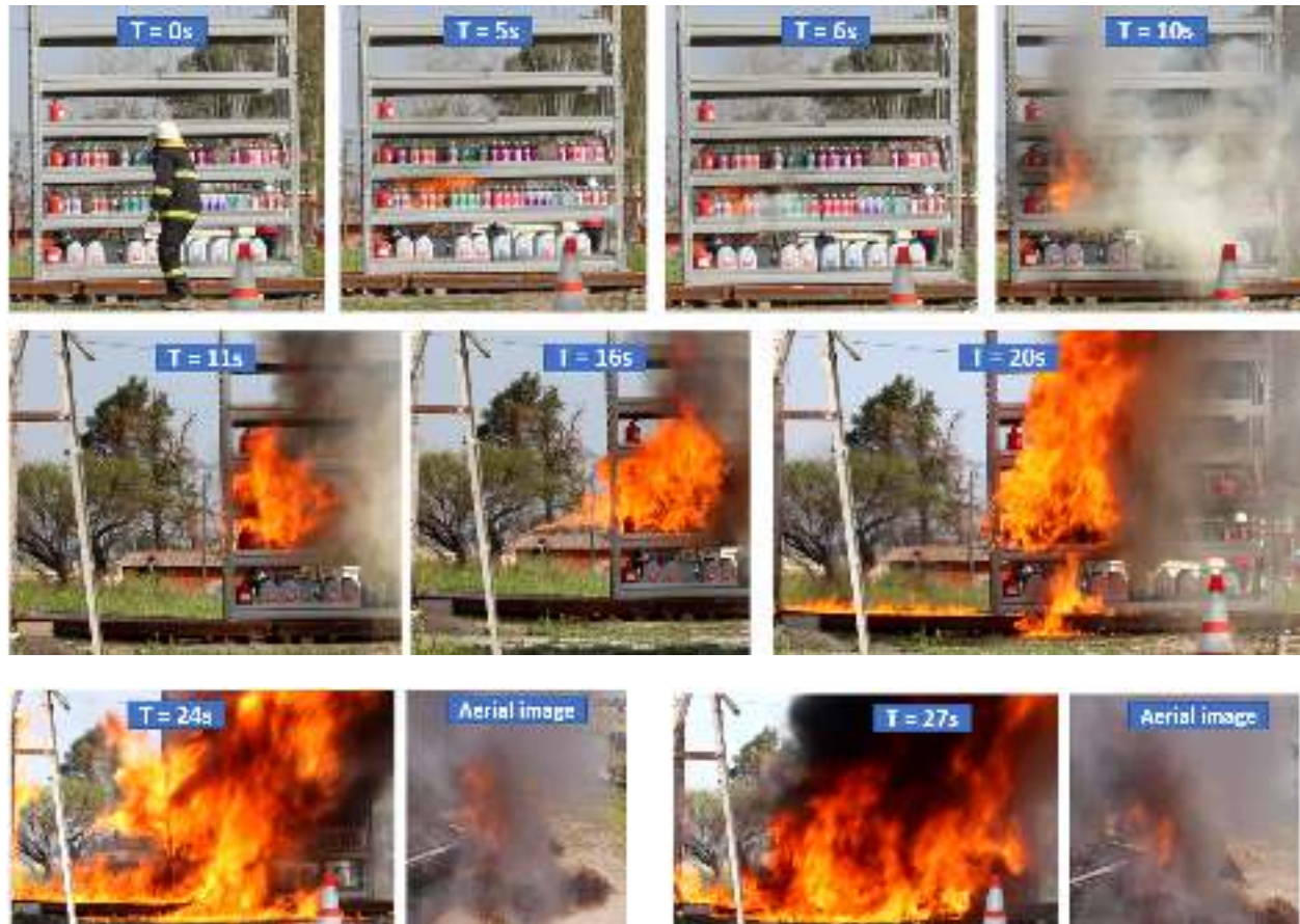
Figure 6: Timeline of the full scale fire test conducted, including the dry chemical system.
