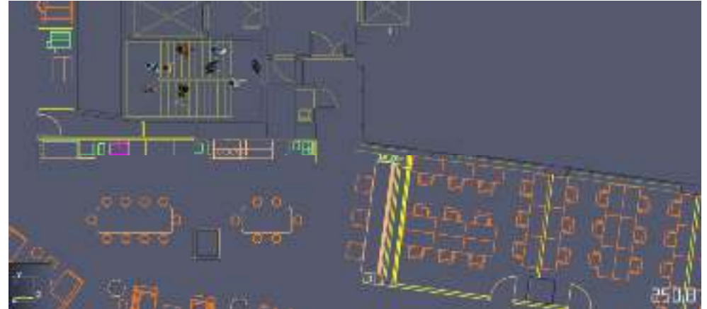
View of the Pathfinder simulation with [speed, size]=[1 m/s, 0.4 m] at t=250 s, floor 6, staircase A
