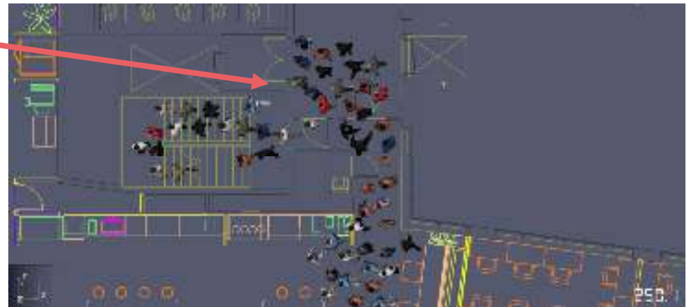
View of the Pathfinder simulation with [speed, size]=[1 m/s, 0.6 m] at t=250 s, floor 6, staircase A
