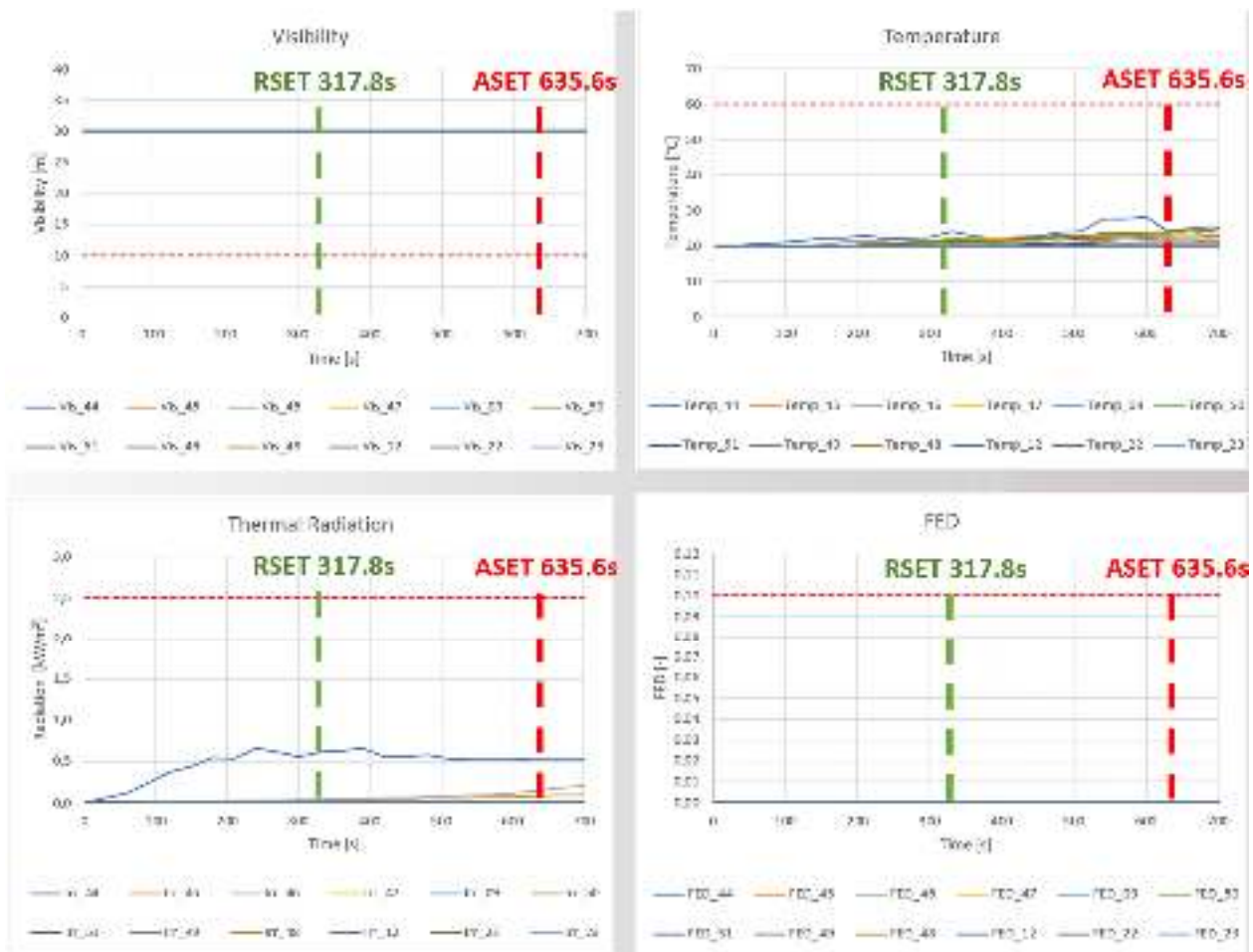
Figure 1: ASET verification of the four monitored parameters: ASET to verify corresponds to RSET obtained from Pathfinder with a margin of 100% of RSET. All four monitors must be below the thresholds until the ASET time is reached.
