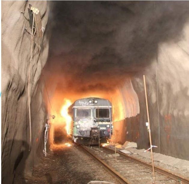
Fire test in the Brunsberg tunnel
