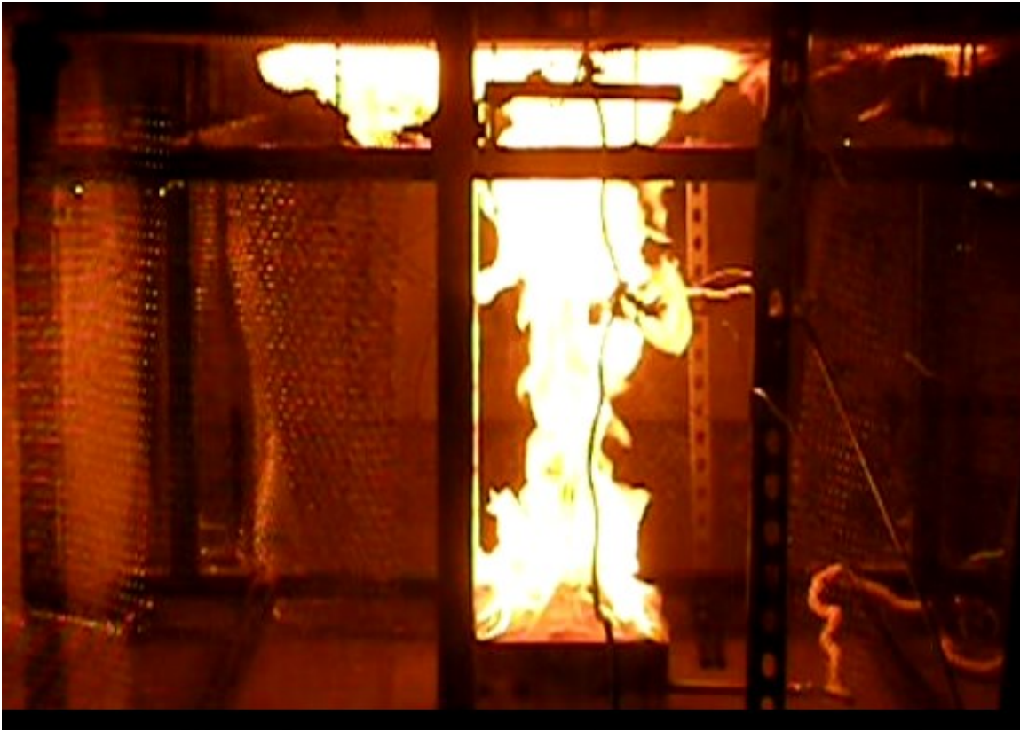
Figure 2: Wasson fire impinging on an unconfined ceiling [27].
