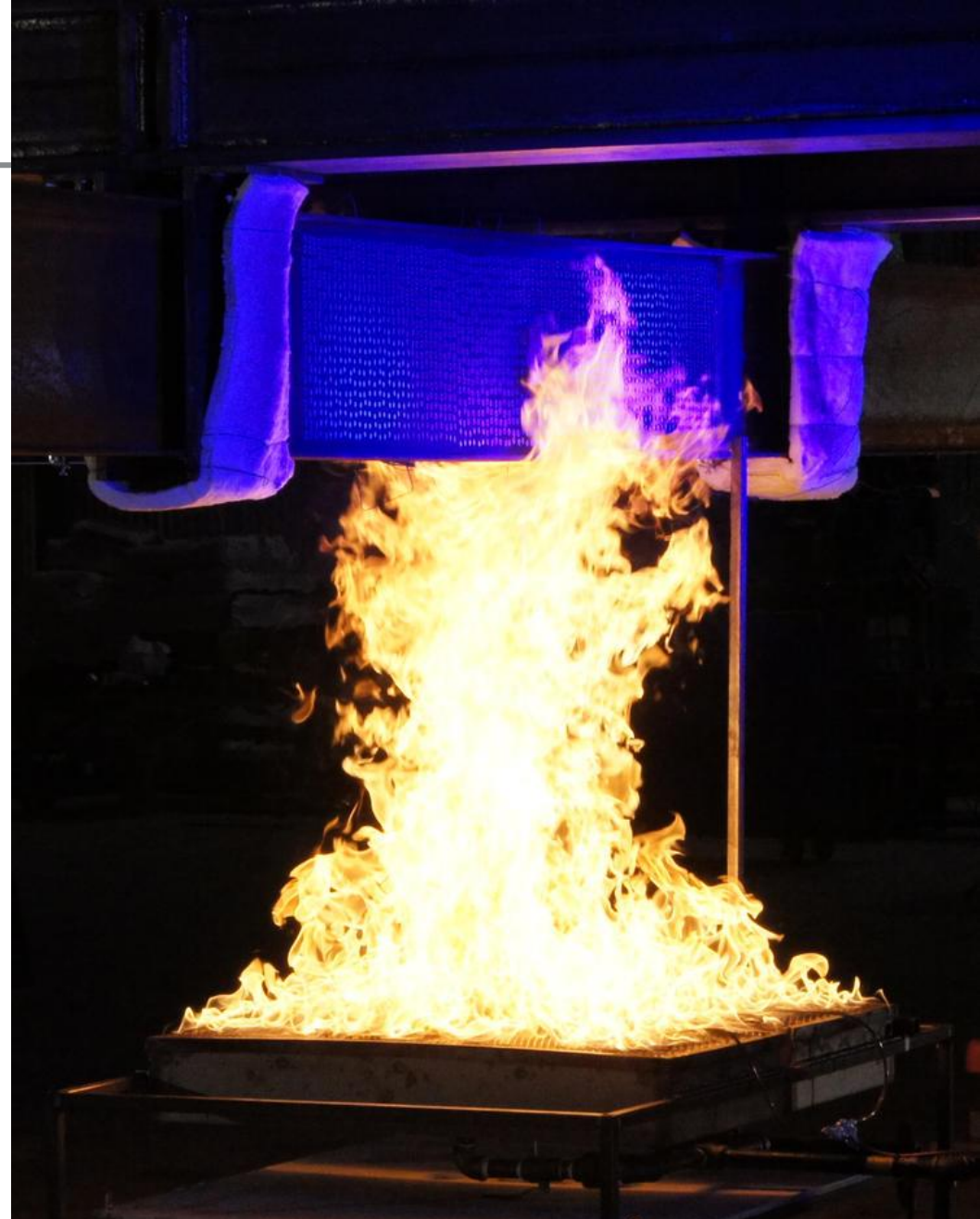
“Behavior of Steel Beams under Localized Fire Exposure”, NIST.
