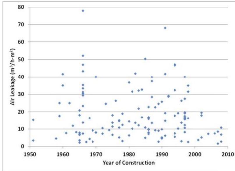
**Figure 5. Building Air Leakage Rate vs. Year of Construction [Emmerish and Persily [2014]**
