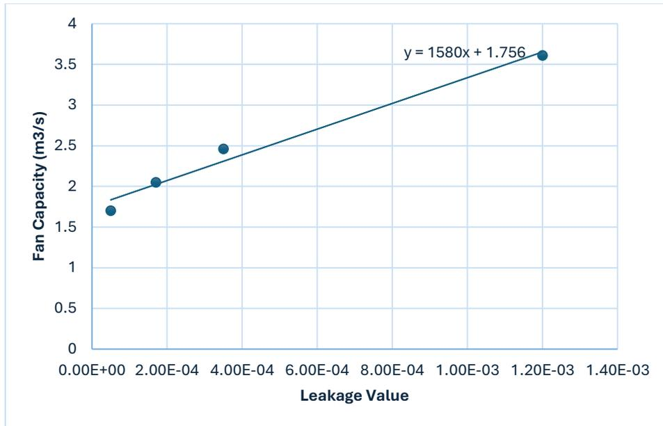
**Figure 7. Stairwell Pressurization Fan Capacity vs. Leakage Rate for Exterior Wall**
