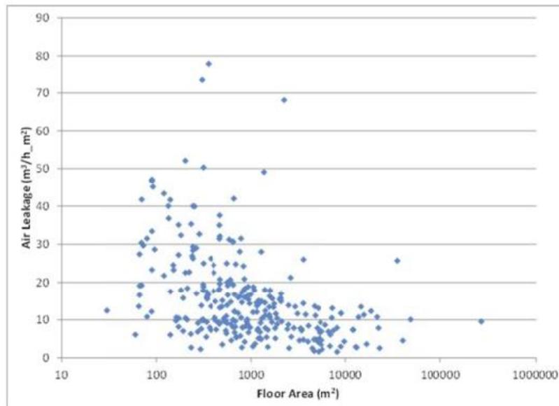
**Figure 2. Building Air Leakage Rate vs. Floor Area of Building [Emmerish and Persily, 2014]**
