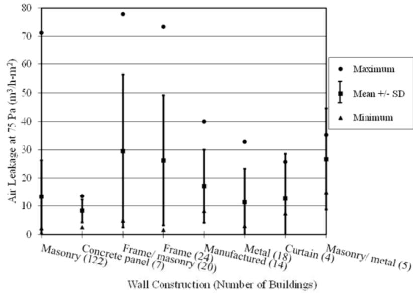
**Figure 3. Building Air Leakage Rate vs. Composition of Exterior Wall [Emmerish and Persily, 2014]**
