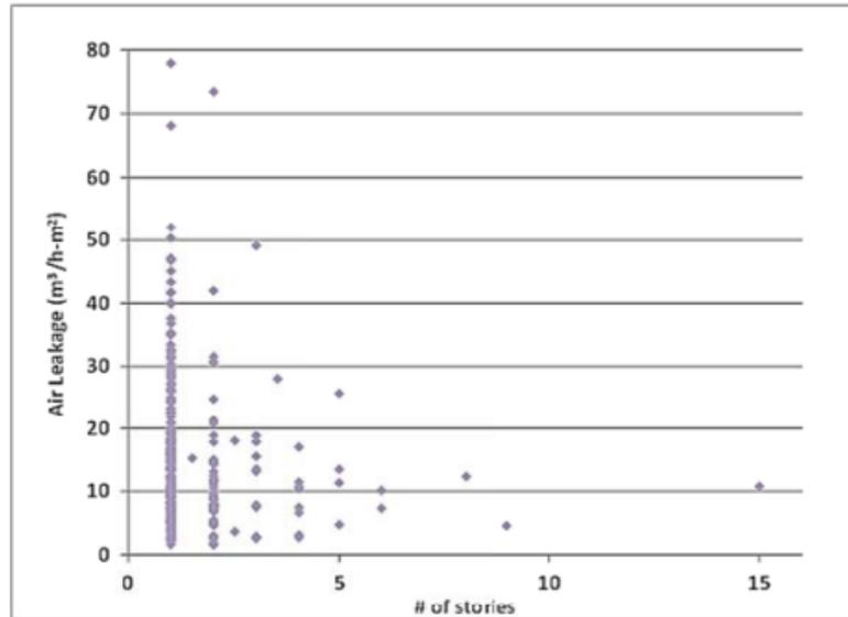
**Figure 1. Building Air Leakage Rate vs. Height of Building [Emmerish and Persily, 2014]**
