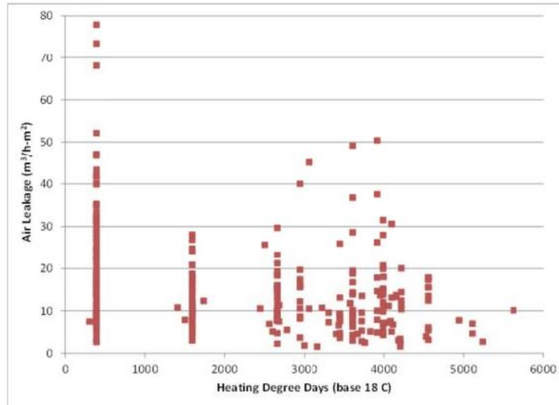
**Figure 4. Building Air Leakage Rate vs. Climatic Conditions for Building Location [Emmerish and Persily, 2014]**
