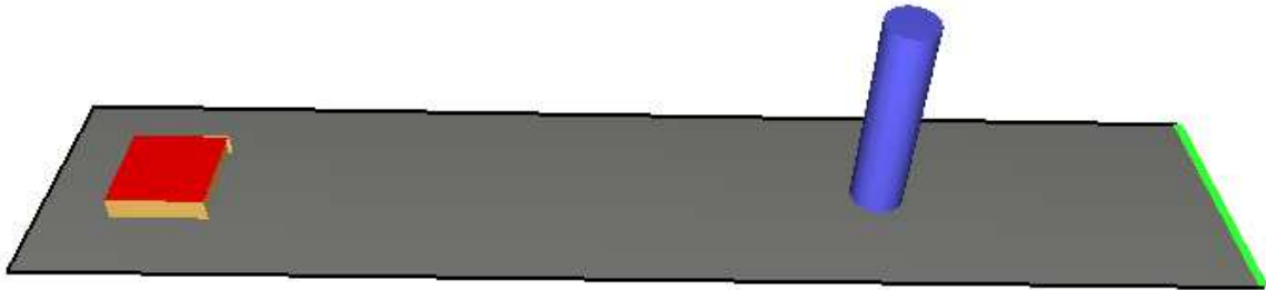
Figure 101. Pathfinder model of FED calculation using stationary occupant.
