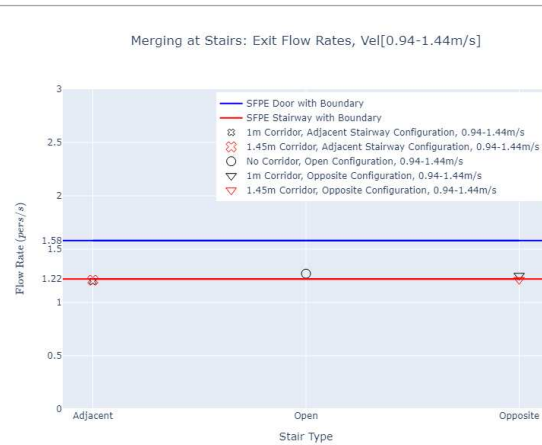
Figure 90. Exit flow rates for stair merging with a uniformly distributed maximum occupant speed of 1.19 \pm 0.25 m/s.
