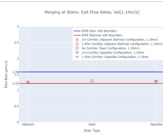
Figure 88. Exit flow rates for stair merging with a constant maximum occupant speed of 1.19 m/s.
