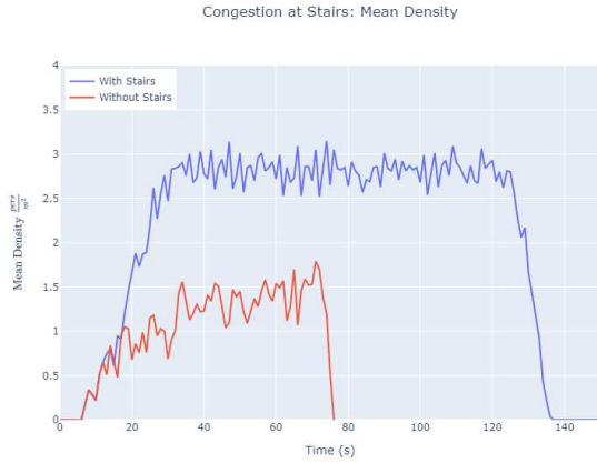
Figure 147. Comparison of mean density at base of stairs with and without stairs.
