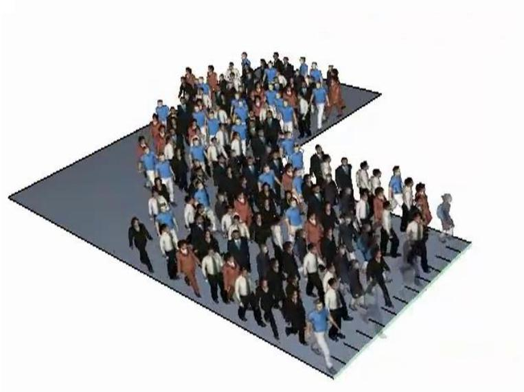
**Fig. 2.** A Pathfinder simulation where a large group turns a corner, then exits through a series of turnstiles.
