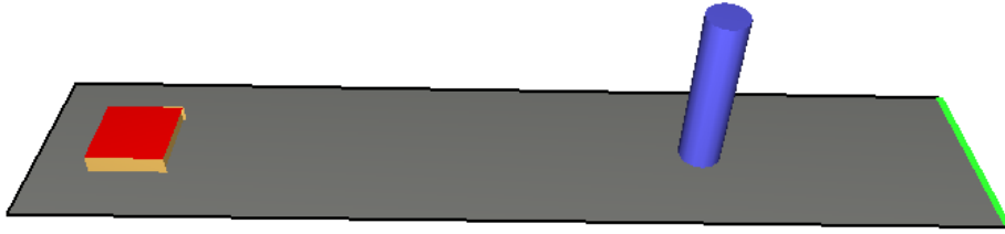
Figure 71: Pathfinder model of FED calculation using stationary occupant.
