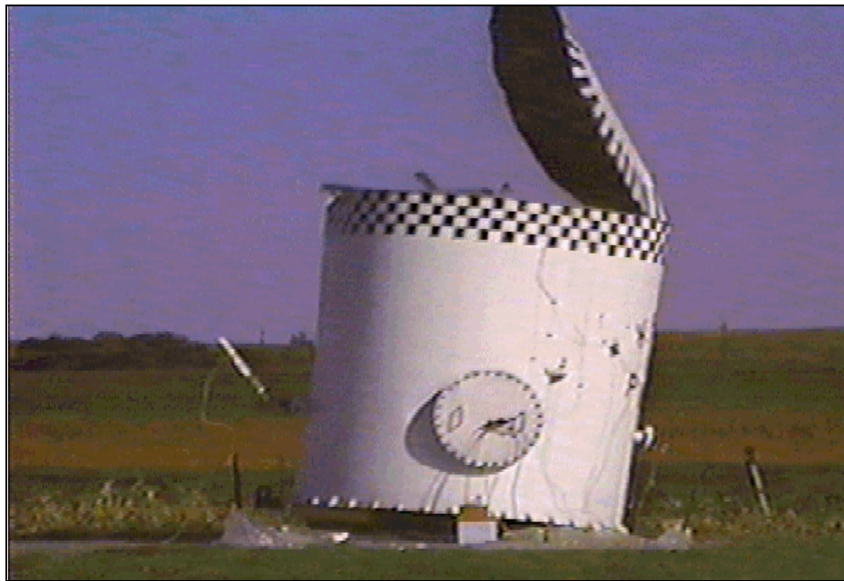
Figure 5.18: Continuously Welded Tank During Test
