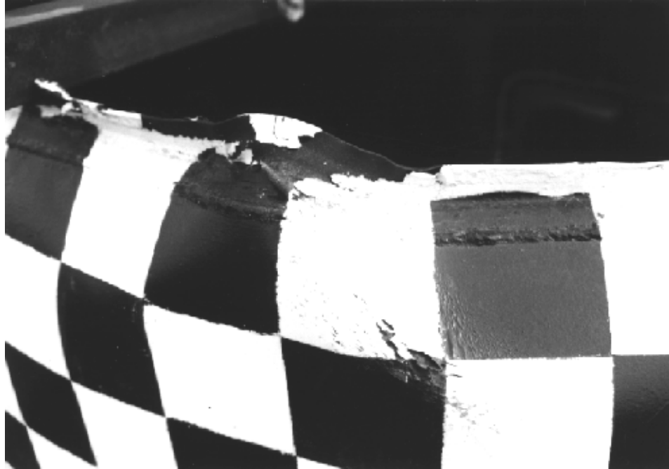
c: Buckled Shell and Angle at Failure Initiation
